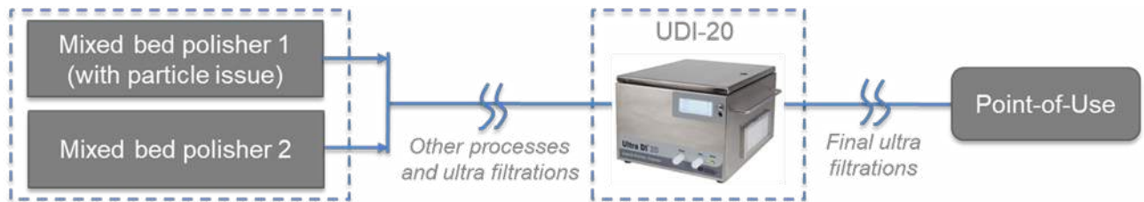
FIGURE 5 MONITOR SCHEME OF MIXED BED POLISHERS & PARTICLE COUNTER
